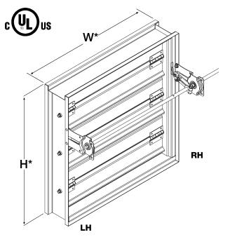
\*W & H dimensions furnished approximately 1/4 in. (6mm) undersize. (Add sleeve thickness for overall sleeved damper dimension) Right hand drive is shown. Left hand drive is available upon request.
